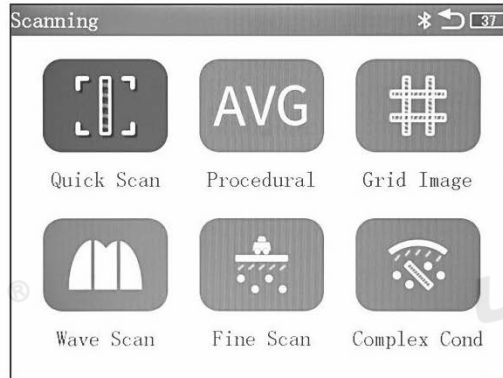
Figure 3.2 Main Interface for Rebar Detection
