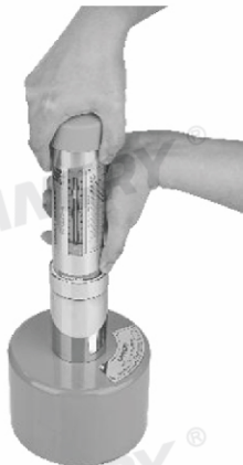
Fig. 3.1 Performance check of the concrete test Hammer (model RH225-A/HT225-N shown)
