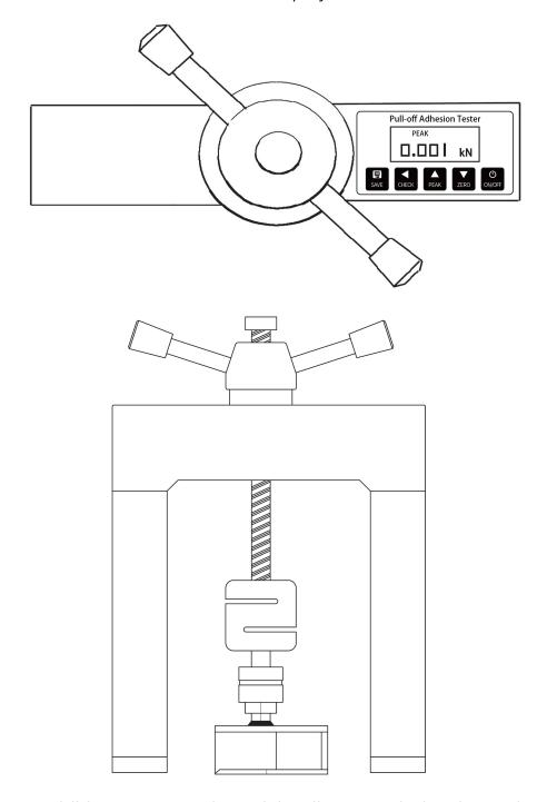
In addition to a set of special pull-out tools for rivets, the tester is also equipped with a set of standard bonding test blocks with specifications of 40mmx40mm and 100mmx100mm.
